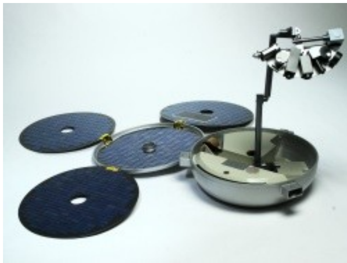
A photograph of the fully deployed Beagle 2. © Beagle 2.
